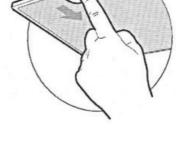
When fitting the filters into the hood pay attention that they are mounted in correct position the handle facing outwards.
