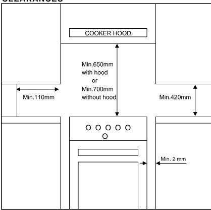
This cooker may be fitted flush to the base units. Leave a gap of approximately 2mm minimum from any adjacent cupboard or appliance. Any adjacent surface must be heat resistant to 50°C above room temperature and if it is higher than the appliance it must be a minimum of 110mm away from the appliance. Any such adjacent cupboard less than 110mm away horizontally, must be at least 420mm higher than the hotplate level.
