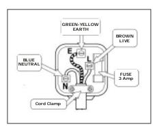
As the colours may not correspond with the markings identifying the terminals in your plug proceed as follows. The green and yellow wire must be connected to the terminal in the plug, which is marked with the letter E, or with the earth symbol or coloured green and yellow. The blue wire must be connected to the terminal marked N. The brown wire must be connected to the terminal marked L.
